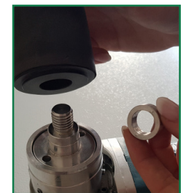
Attention: remove the spacer ring for models Bosch, Makita, Metabo and Milwaukee
